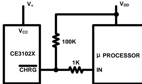
Figure 7. Using a Microprocessor to Detect  $\overline{\text{CHRG}}$  State
