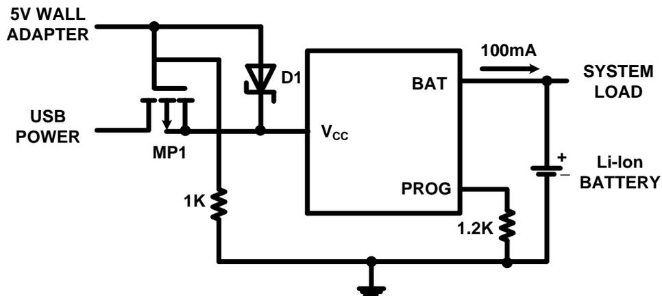
Figure 9. Combining Wall Adapter and USB Power
