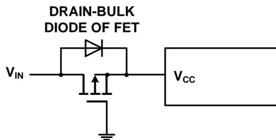
Figure 8. Low Loss Input Reverse Polarity Protection
