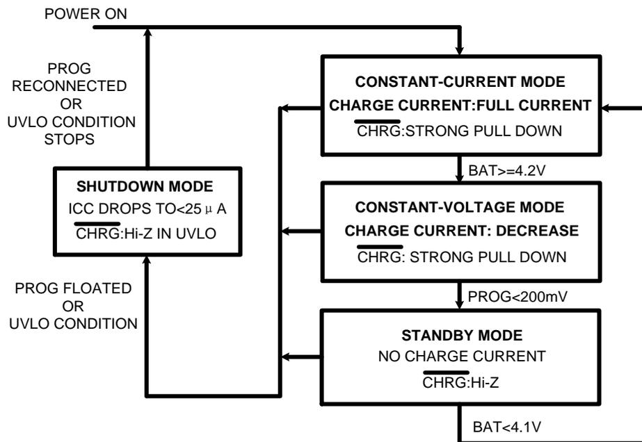
Figure 3. State Diagram of a Typical Charge Cycle
