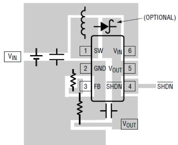
RECOMMENDED COMPONENT PLACEMENT. TRACES CARRYING HIGH CURRENT ARE DIRECT. TRACE AREA AT FB PIN IS SMALL. LEAD LENGTH TO BATTERY IS SHORT.
